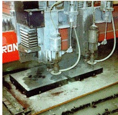
water jet cutting with a double head
